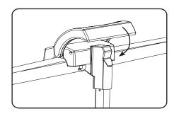
**6.** Extend the Support Rod to the desired viewing position and lock into place. The screen can be levelled using the adjustable feet.
