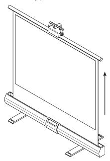
**5.** Lock the screen onto the support rod with the handle
