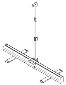
**4.** Pull the screen up and hook into the top of the support rod.
